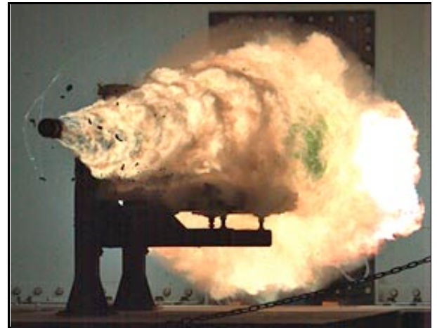
A high-speed Navy video image showed a projectile as it was shot from an electromagnetic railgun at Mach 7 in a test Thursday in Dahlgren, Va.
