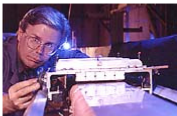
The scale model needs to achieve higher takeoff speeds than a full-size train.
