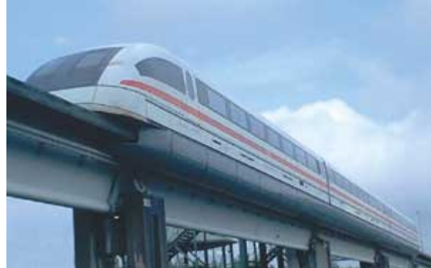
MAGLEV TRAIN - The 'Transrapid' German magnetic levitation passenger train at a test facility in Emsland, Germany.
